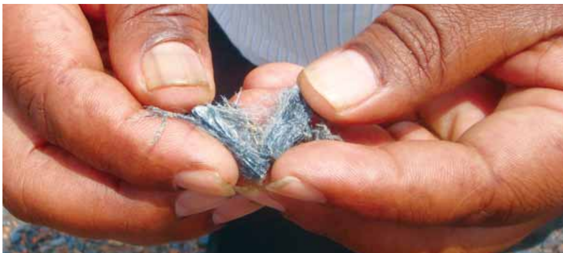
A close-up of crocidolite from the Kuruman area. The fibres visible here are approximately 6 000 times longer than regulated fibres Photo courtesy of Jim teWaterNaude
